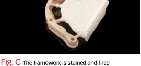
FIg. C The framework is stained and fired while still connected to a piece of the block.
