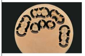
Fig. 1 Aesthetic Press Vanilla wax blank with the milled units. The blank is available in different sizes as 14,16,18,20,25, and 30 mm
